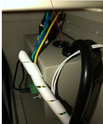
Hardwiring feed through hole
